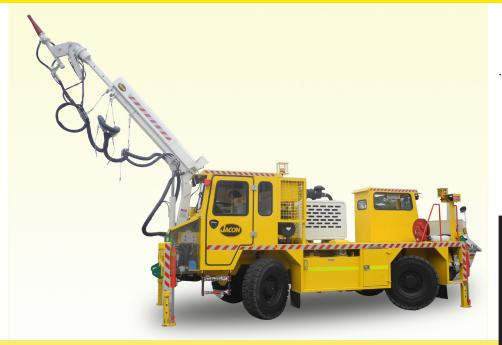
THE JACON MAXIJET X3 IS A MID-SIZED SHOTCRETE RIG DESIGNED AND BUILT FOR TRAMMING IN HARSH CONDITION. STEEP INCLINES AND LONG DISTANCE.
