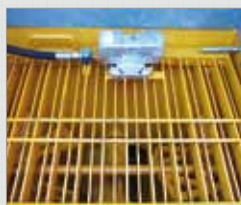
4 Hopper designed for concrete spraying
